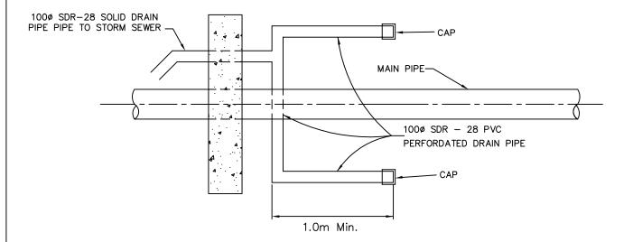
DRAINAGE PIPE ARRANGEMENT.
