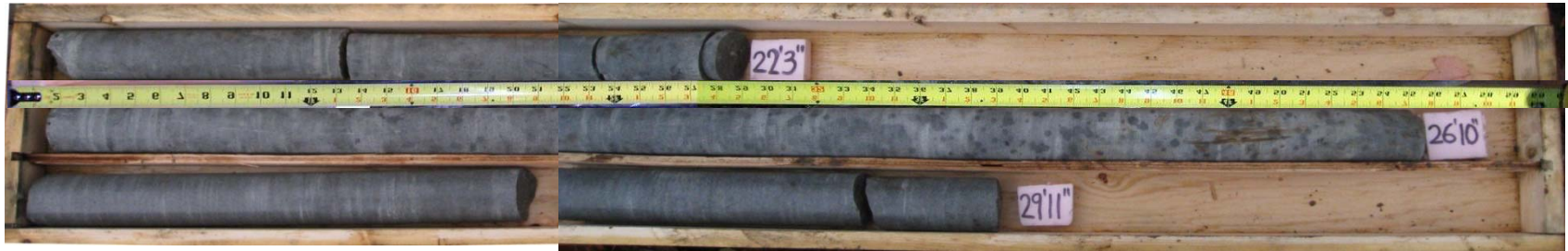
BH10-06 – Box 1 of 1: 5.6 m to 9.1 m (18'5" to 29'11")
