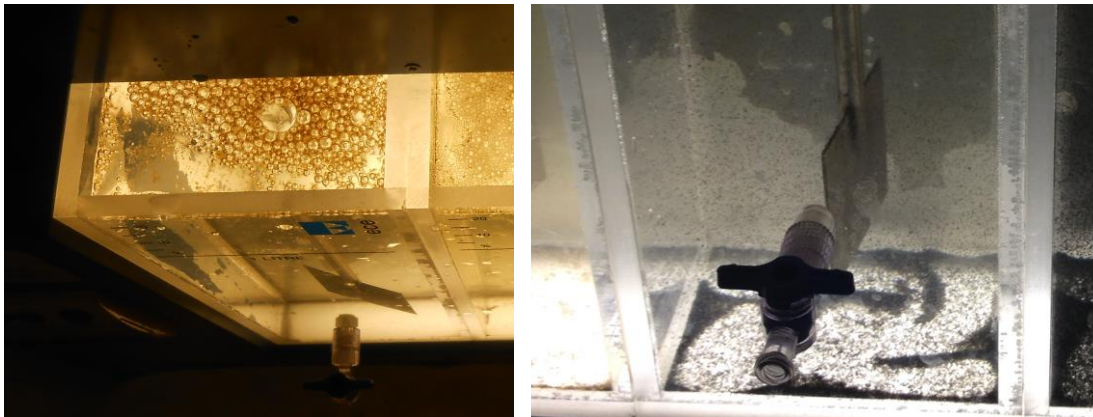
Figure 1-3 and 1-4: Typical float (ClearPAC, 15 mg/L) and settled floc (alum + PAC)
