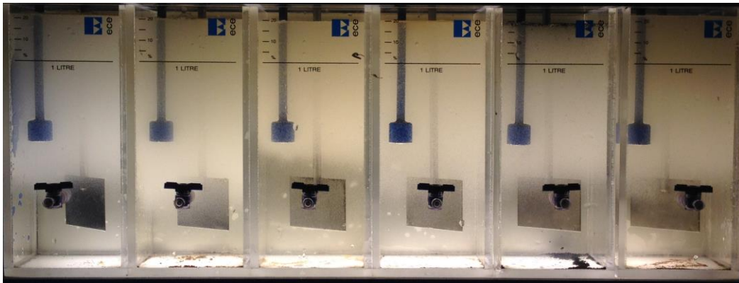
Figure 1-2: Bubbles being released during DAF
