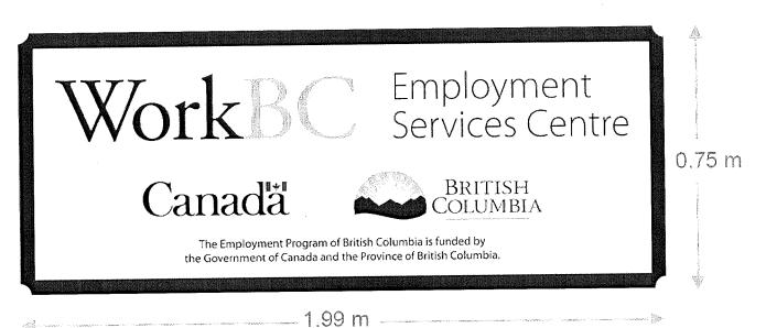
Sign construction: 1.5 sq.m. aluminum sign with vinyl face
