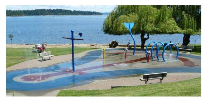
The rubberized surface is in generally good condition, but the expected useful life of the surface may be reduced due to the high amount of sand that gets tracked in from the beach and abrades the surface. Water from the spray park is reclaimed for irrigation, but is left untreated. This was permitted in the past, but current health regulations may require future upgrades that provide for above ground re-use of water to have treatment, which comes with a high capital and ongoing operating cost.
