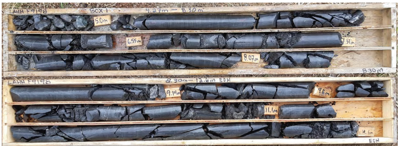
Photo 2.4.4 – Rock Core Samples, BH21-02 from 4.27m to 12.65m
