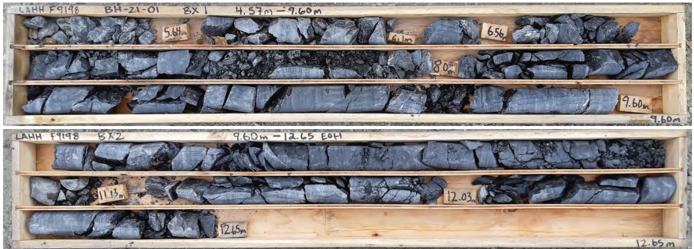
Photo 2.4.3 – Rock Core Samples, BH21-01 from 4.54m to 12.65m
