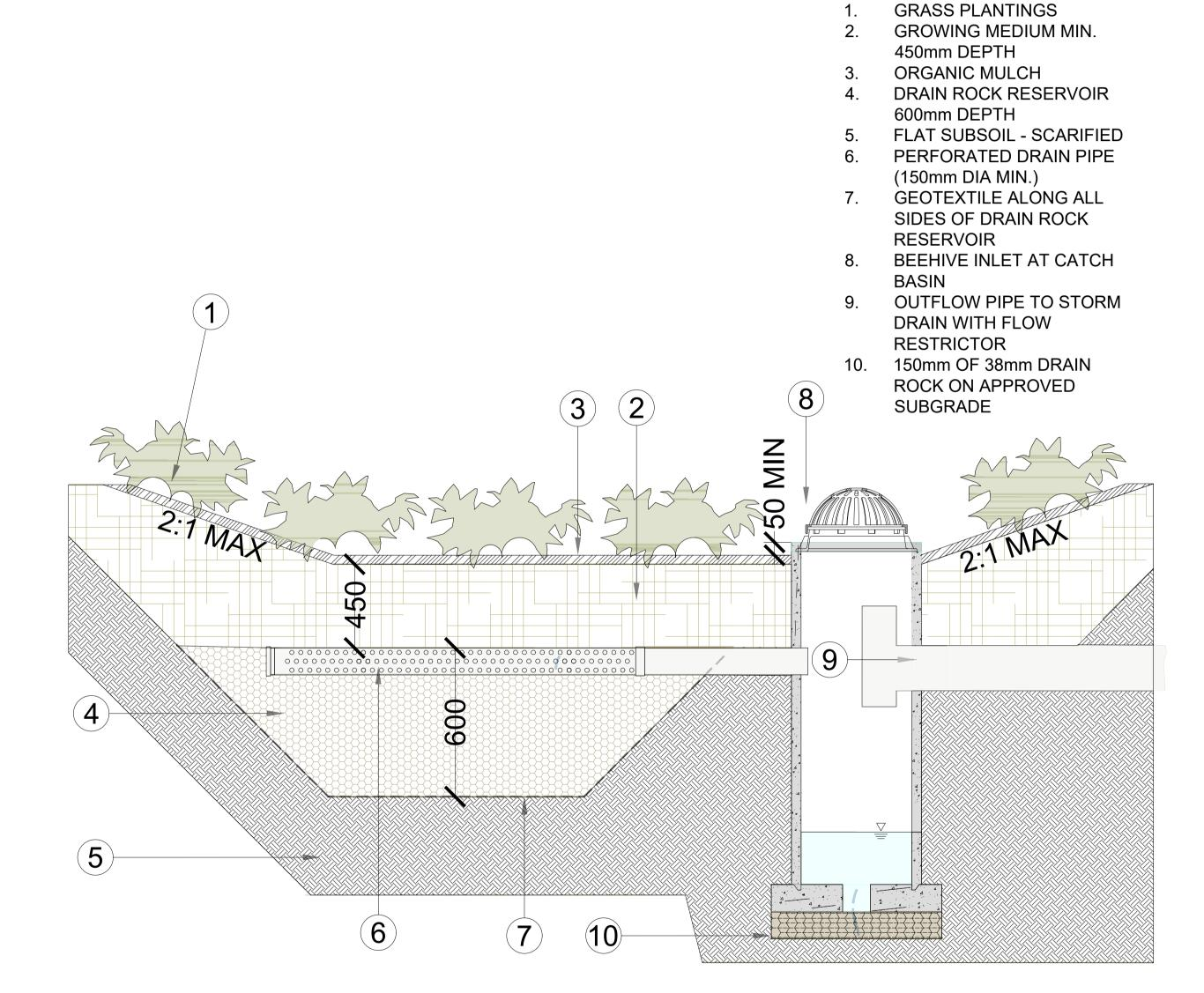
RAIN GARDEN — PARTIAL INFILTRATION. MODIFIED FROM STORMWATER SOURCE CONTROL GUIDELINES 2012. NTS.
