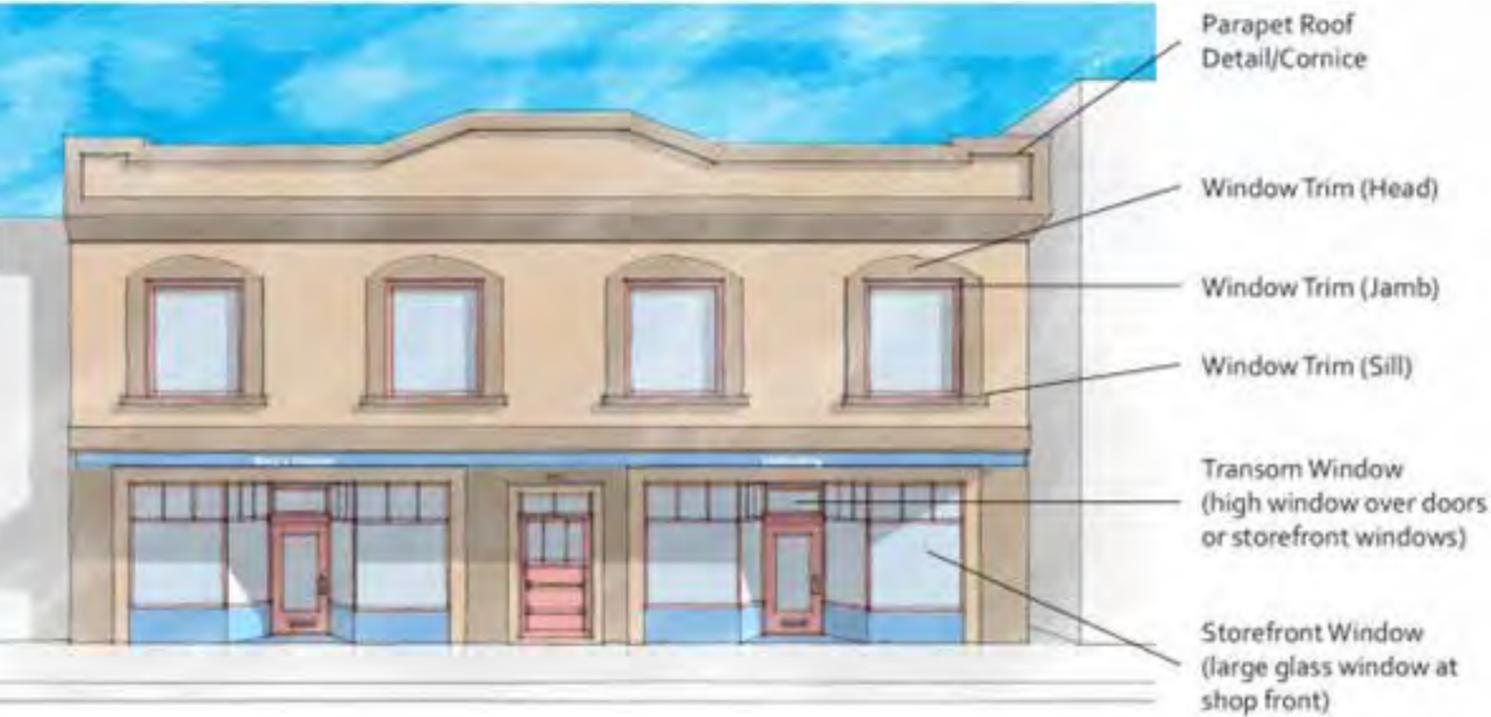
Window, door, and roof details to incorporate in commercial buildings.
